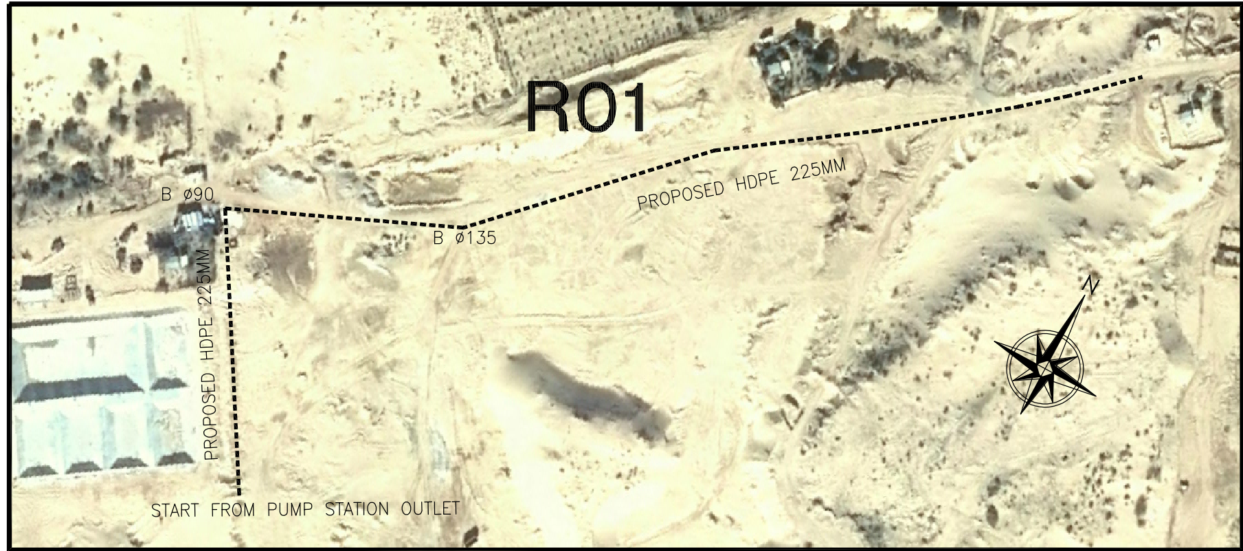
PLAN FOR R01 FROM St. 0 to St. 50 SCALE: 1:1000
